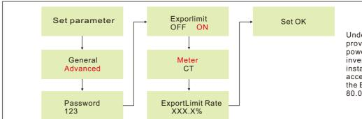
Under the permission given by your energy provider, the ratio of your system output power divided by the rated power of the inverter is called Export Limit Rate. For instance, if the energy provider only accepts 2.4kW from your 3kW system, then the Export Limit Rate of 3kW inverter is 80.0%.
