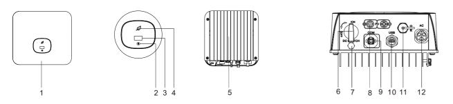
(1)Front panel (2)Touch button (6)DC switch (7)Vent valve (3)OLED screen (8)PV terminal (4)LED indicator (5) (9))COM port (10
